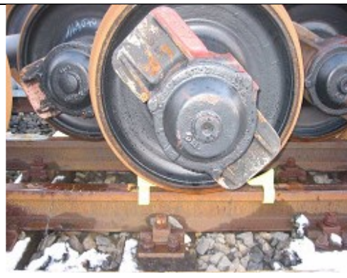
Photo 2: Storing in staggered formation on track using safety scotches
