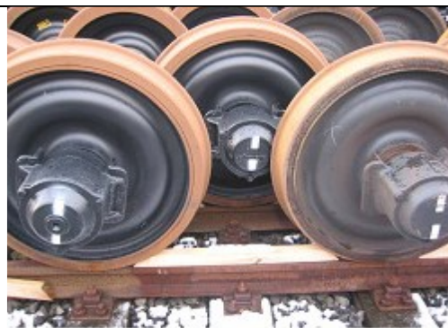
Photo 3: Storing in staggered formation (with double rail)
