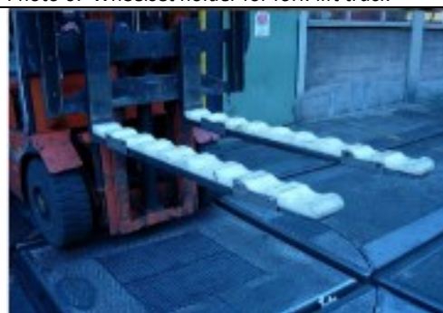
Photo 8: Wheelset holder for fork-lift truck (several wheelsets)
