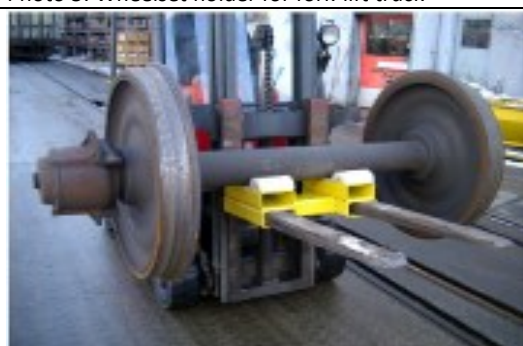
Photo 7: Wheelset holder for fork-lift truck (loaded)
