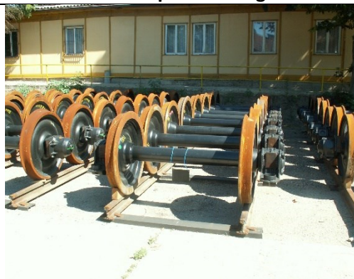
Photo 1: Storing on track using safety scotches
